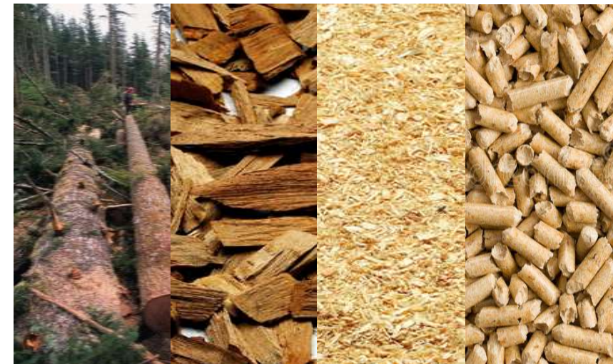
CHIPPING – WET GRINDING – DRYING – GRINDING – PELLETING
