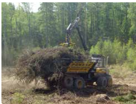
Modern residue gathering equipment in Finland.
