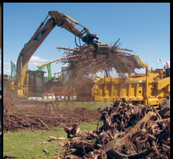
Vermeer crusher shows how it converts branches, tops, and stumps to wood fuel. Photo: Sofie Samuelsson
