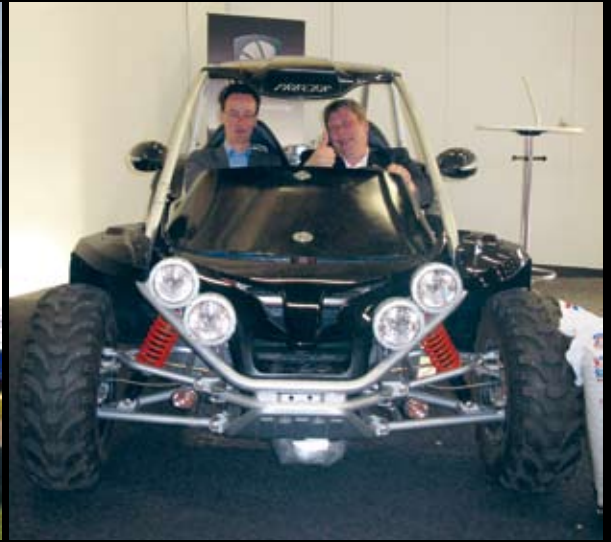
Anders Haaker, editor of Swedish magazine Bioenergi, and Olof Arkelöv from Kanenergi test the first pellet-hybrid car from Precer, which runs on an electric engine powered by a wood pellet-fuelled Stirling motor. Photo: Sofie Samuelsson
